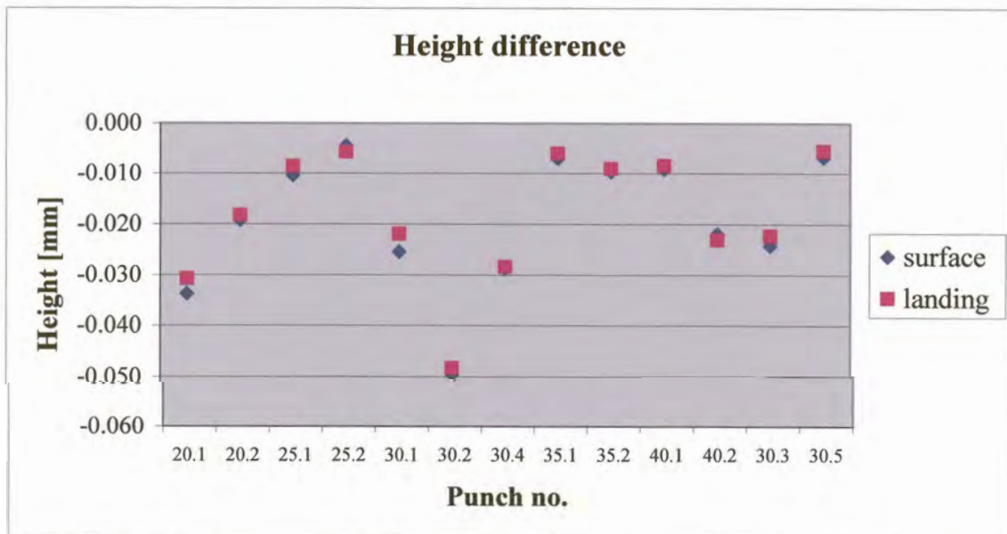
FIGURE 4.32 Difference in height of the landing and design surface after heat treatment.
