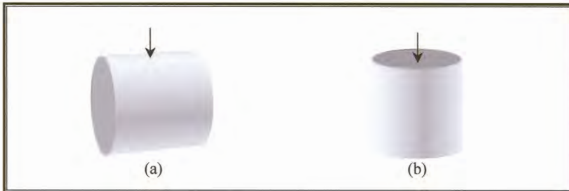
FIGURE 1.16 Measuring point on the (a) outer and (b) inner surface
