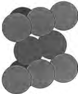
Figure A9. The fcc (110) surface
