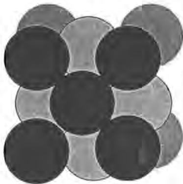
Figure A7. The fcc (100) surface
