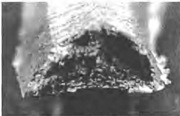
Figure 2.7 Cross section of an aluminium chip showing thick middle section and taper towards sides
