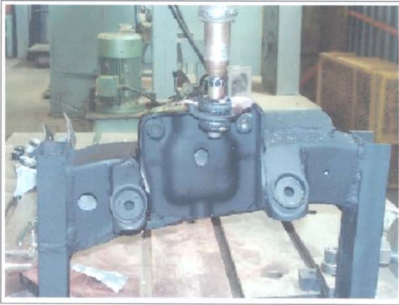
Figure 6.3: Original suspension bracket - 4x4 pick-up truck
