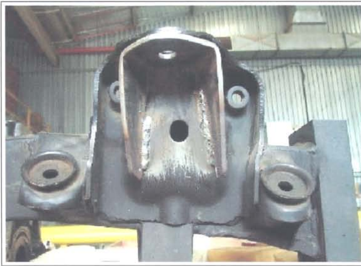
Figure 6.4: Modified suspension bracket - 4x4 pick-up truck
