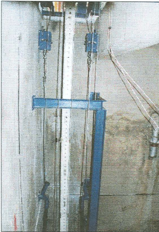
Figure 30 Loaded strips before cage impact.
