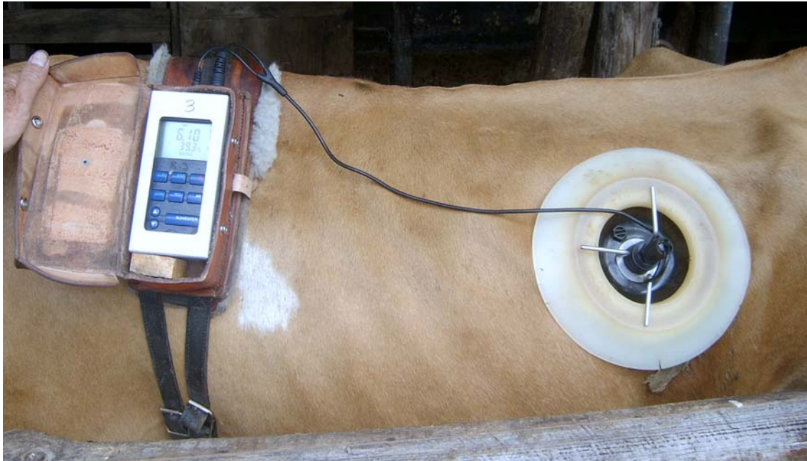
Figure 3.1 Ruminant pH was recorded at 10 minute intervals on a data logger (WTW pH 340i pH meter/ data logger) connected to an electrode (WTW SenTix 41 pH electrode) placed in the rumen via the cannula
