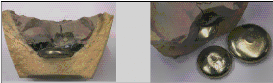
NiS button formed and slag layers above (Chan et al, 2001).
