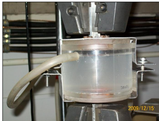
Figure 3.5. The Plexiglas corrosion fatigue chamber.
