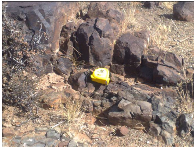
Figure 3.7 Contact between Hansrivier dolerite dyke and host rock (tape measure as scale).
