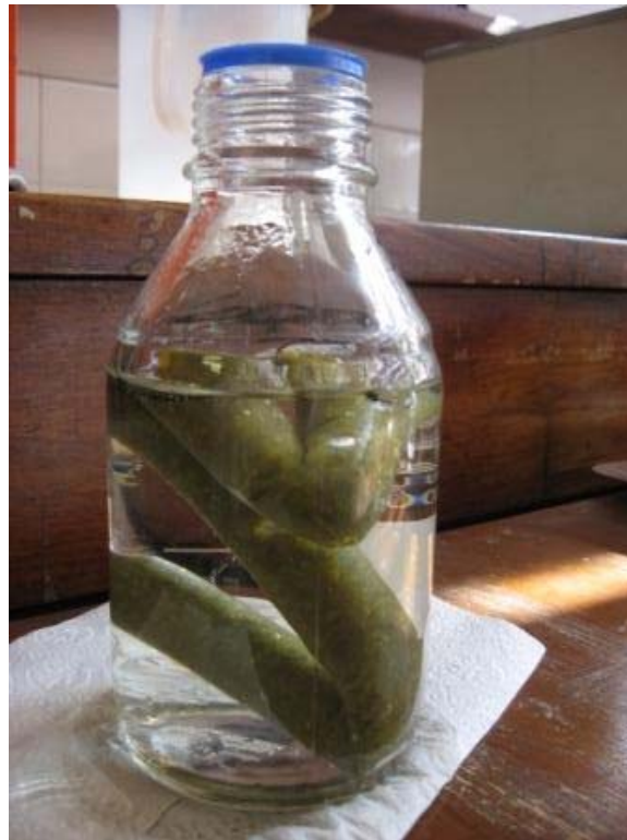
Figure 3.4: Dialysis tubes surrounded by buffer solution during the small intestinal phase
