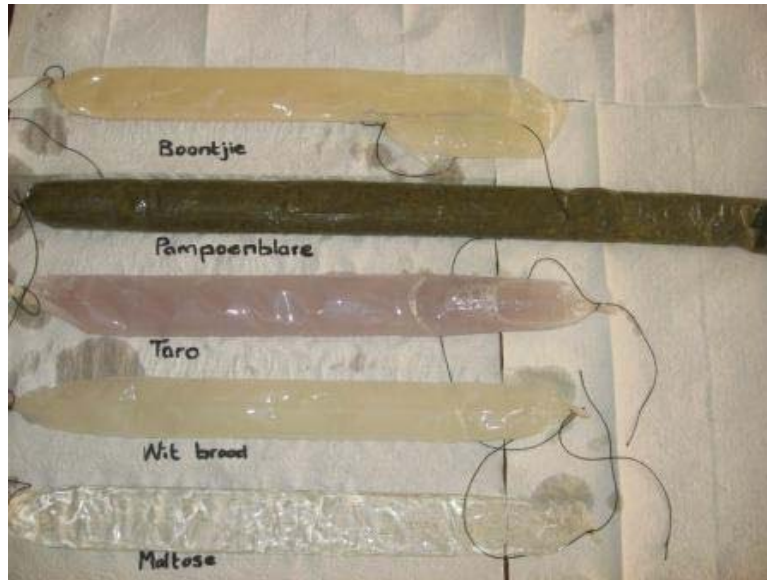
Figure 3.3: Dialysis tubes containing the food samples, representing the small intestinal phase
