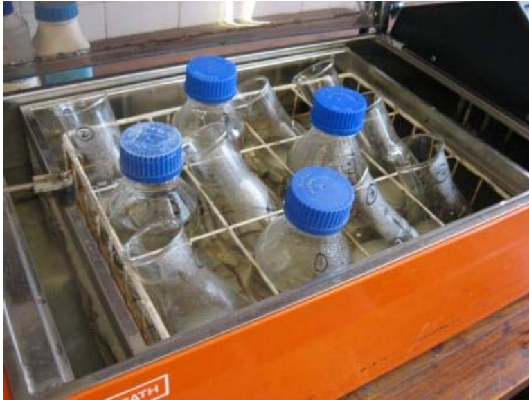
Figure 3.2: Samples in the shaking water bath at 37°C for one hour during the gastric phase
