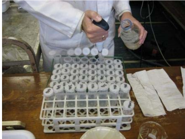
Figure 3.5: Transfer of buffer solution from a flask to containers for the analysis of amount of carbohydrate which diffused through the dialysis tube into the surrounding fluid.
