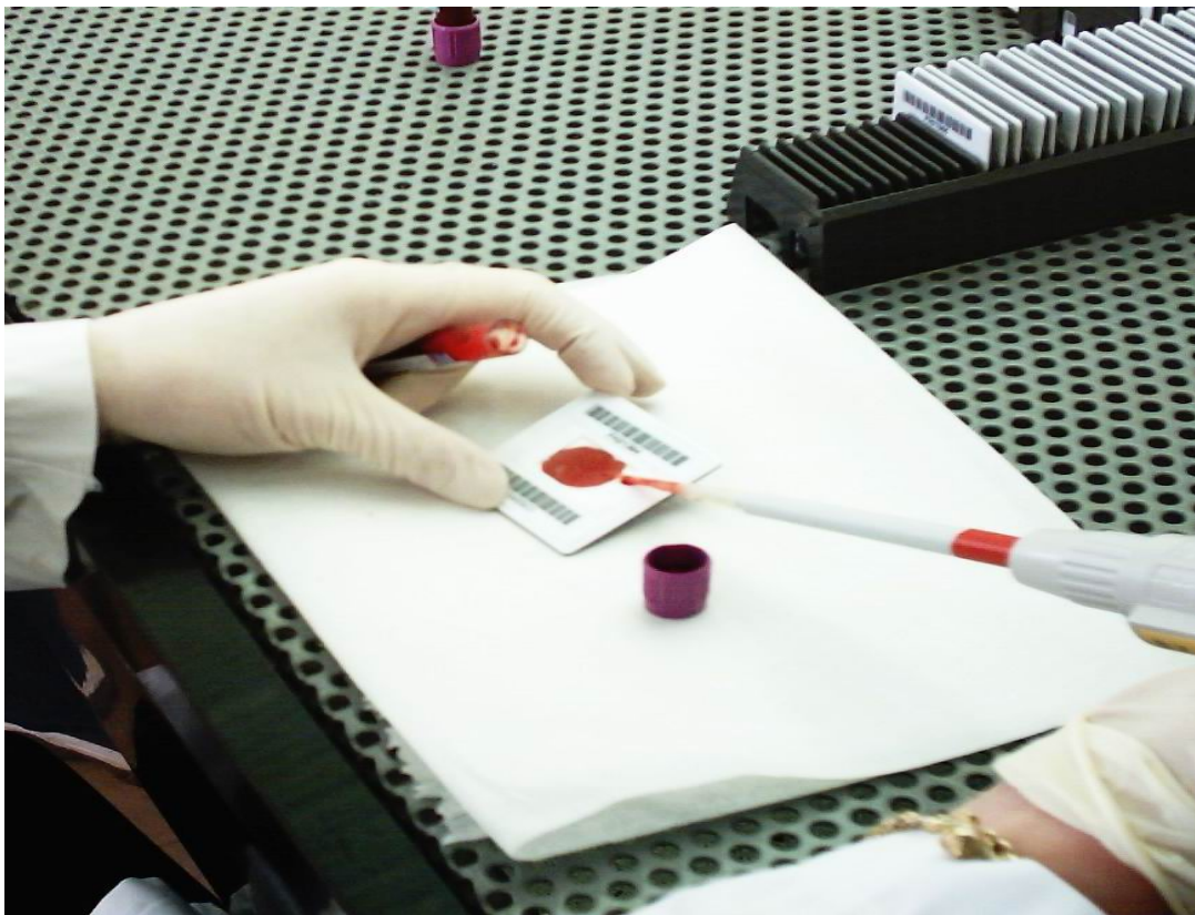
Figure 3.2: Spotting blood from EDTA vacutainer ™ tubes into a barcoded FTA ® paper slide under a fume- hood
