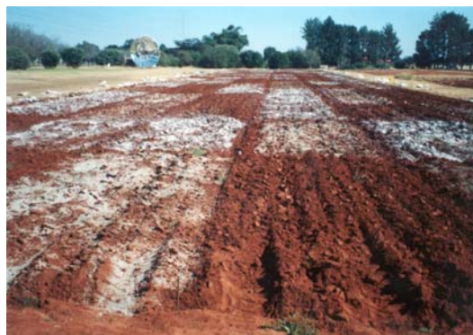
Figure 1: Class F Fly ash, SLASH and lime treated field trial at the Hatfield Experimental Farm, University of Pretoria.
