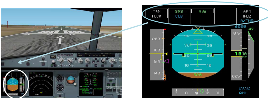
Figure 3.3: Modern Primary Flight Display (PFD) with Flight Mode Annunciator (FMA)
