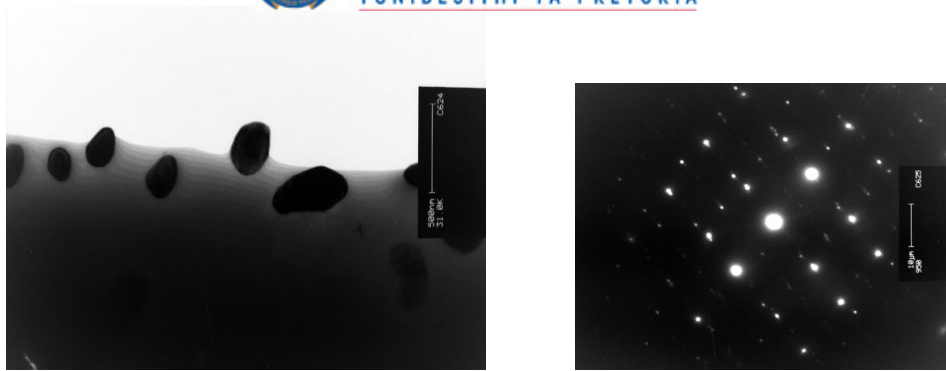
Figure 8.10. Transmission electron micrographs and corresponding selected area diffraction (SAD) pattern from Steel A annealed at 750 °C.
