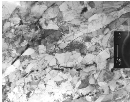
Figure 6.13. TEM micrograph showing the presence of a dislocation substructure and some fine Laves precipitates in the as received hot rolled specimen of Steel A, indicating a lack of full dynamic recrystallisation during the last stage of hot rolling.
