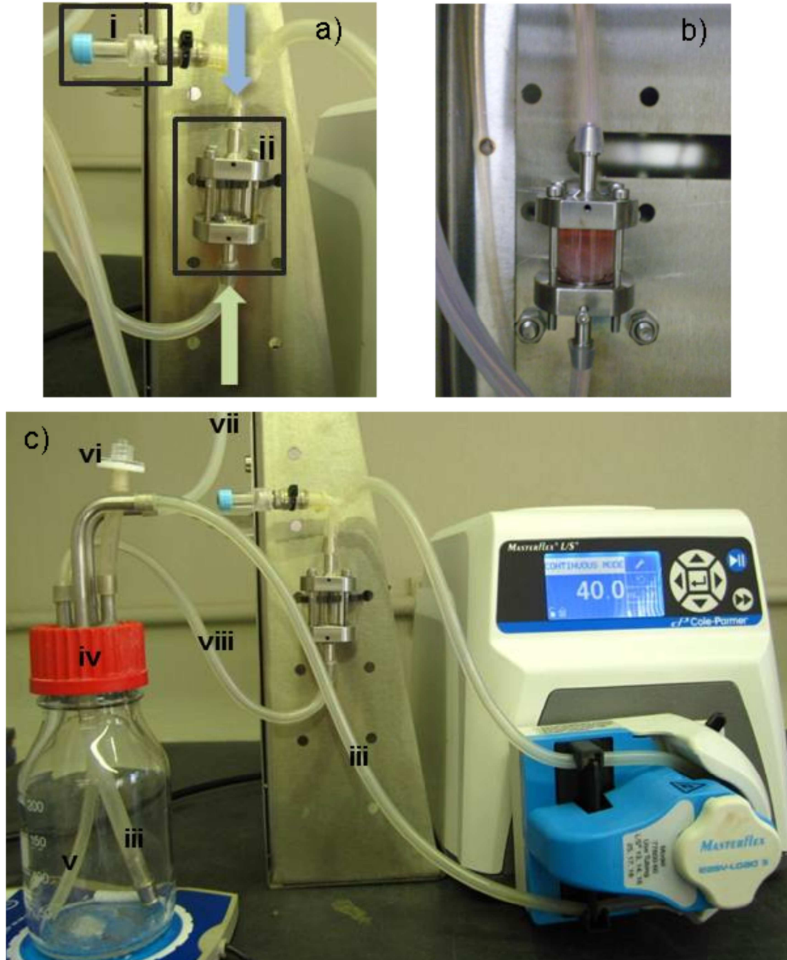
Figure 6.2: Preliminary prototype of the CSIR's T3D showing (a) i) sampling port through which cells are injected into the bioreactor; and ii) small volume bioreactor (without scaffolds); (b) close-up view of bioreactor containing stacked NWF disks (1.5mm diameter) with cells and media; and (c) full view of the preliminary prototype system showing the peristaltic pump used for pumping iii) media from (iv) media reservoir to the bioreactor; v) gas inlet (into the media); vi) gas vent; vii) gas line from tank; and viii) media return line (from the bioreactor).
