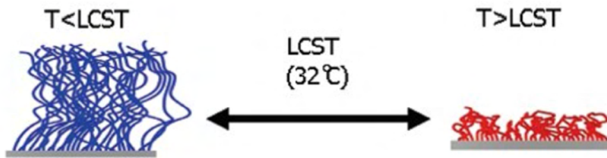
Figure 2.5: Image showing the phase transition of PNIPAAm attached to a surface at temperatures below and above the LCST (Cooperstein and Canavan, 2010).
