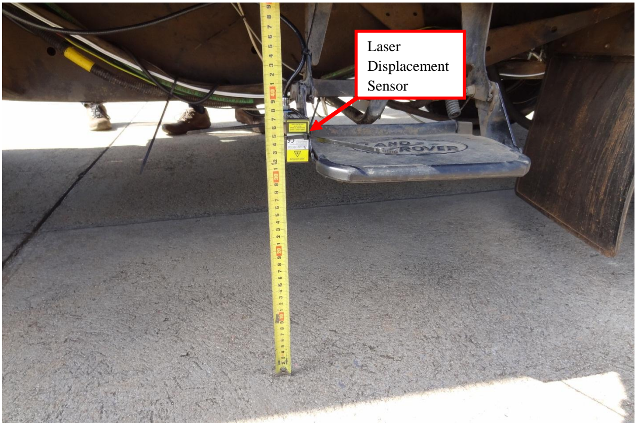
Figure 79 Laser displacement sensor on the side of the vehicle
