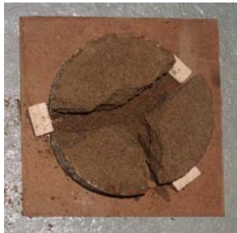
Plate 4.8: Three-plane failure of DPTT specimen
