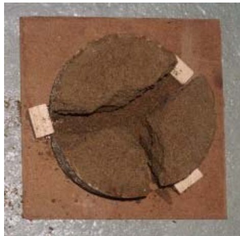
Plate 4.8: Three-plane failure of DPTT specimen
