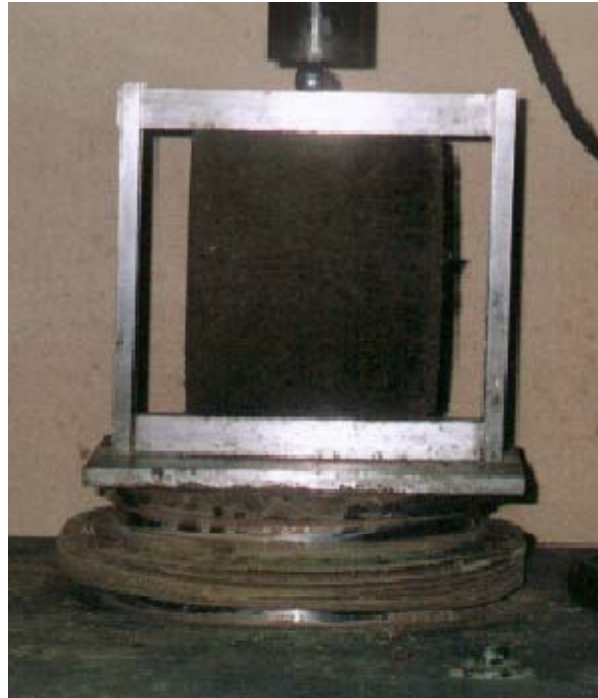
Plate 4.5: Positioning of the test specimen in ITS (Courtesy Africon Labs)
