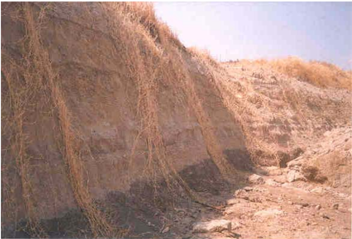
Plate 2.4: Stratification of pozzolanic layers (Mbeya region)
