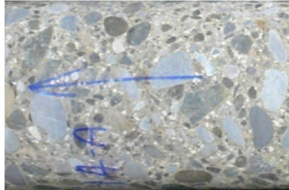
Plate 8.2: Typical RCC Core
