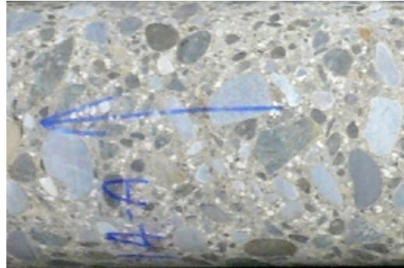
Plate 8.2: Typical RCC Core
