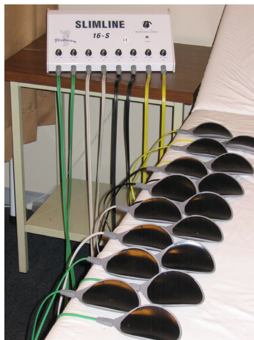
FIGURE 3.8: SLIMLINE ELECTRICAL MUSCLE STIMULATION (EMS) MACHINE
