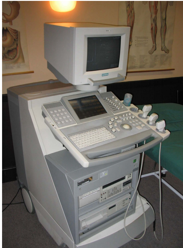
FIGURE 3.6: SIEMENS (SONOLINE ELLEGRA) SONOGRAPH
