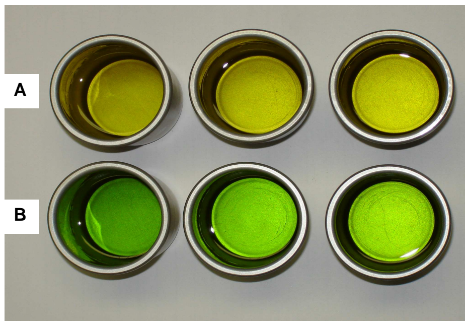
Figure 2.3.3: Appearance of oil extracted from ripe avocado fruit with supercritical carbon dioxide (SC-CO 2 ). A – oil from ripe, oven-dried fruit; B – oil from ripe, freeze-dried fruit.
