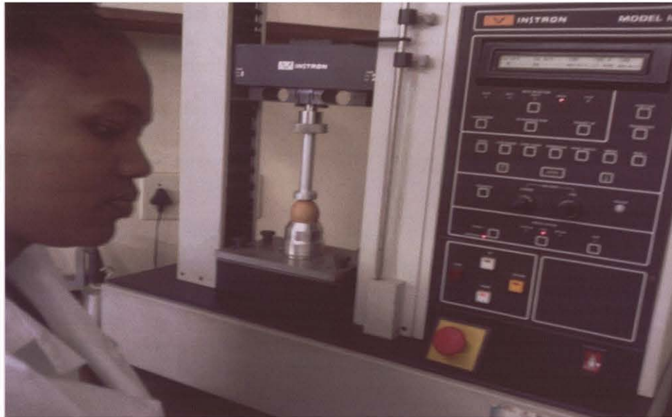
Figure 3.9 Measuring egg shell strength using Instron 10111
