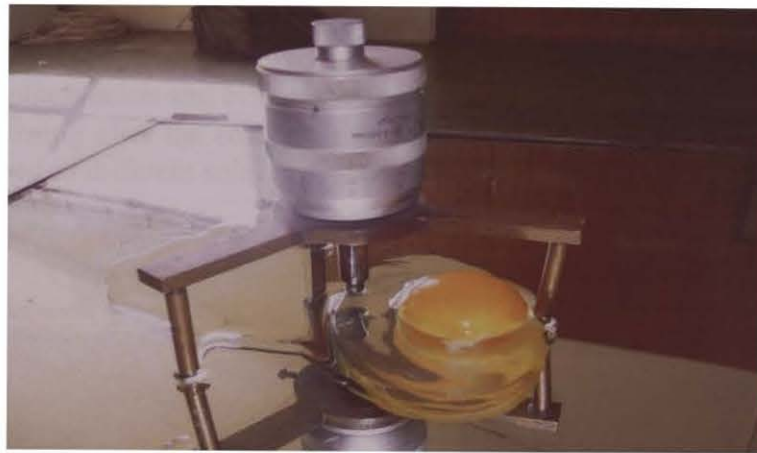
Figure 3.6 Mututoyo gauge for measuring albumen height
