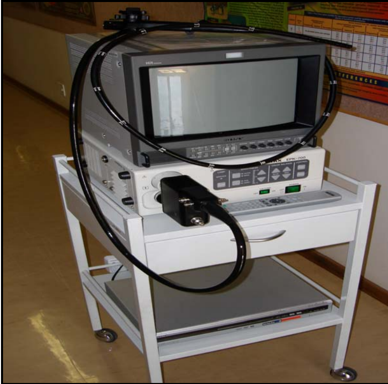
Figure 4.1 The portable flexible videoendoscopy system used in the grading of respiratory tract disorders in South African Thoroughbred racehorses.
