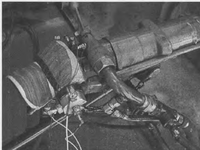
Figure 4.7: Instrumented drill handle showing the tri-axial accelerometer set-up
