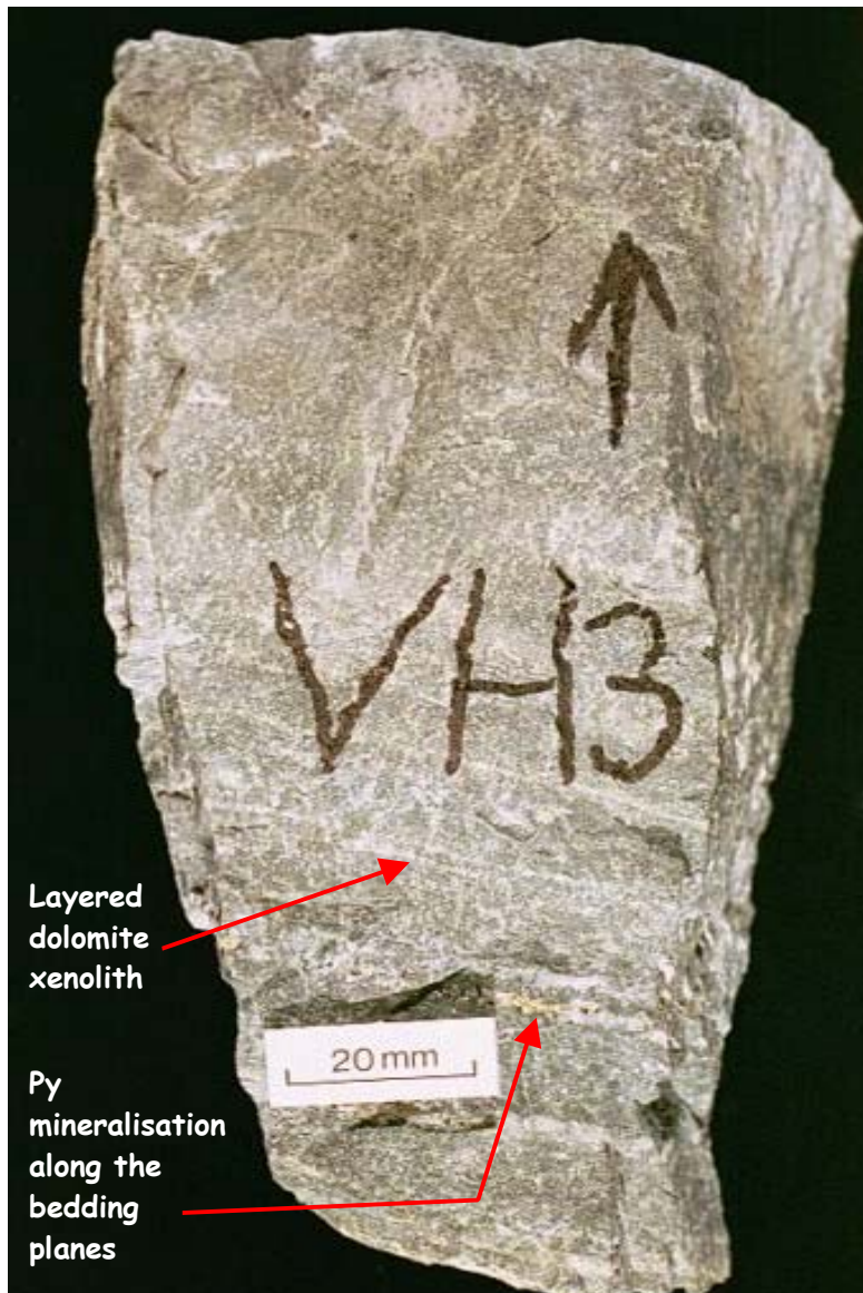
Figure 3. 15: Hand specimen showing pyrite (Py) mineralisation along the bedding planes in the dolomite xenolith. Sample Number: VH3. Bulk Sample Drive, BMZ.
