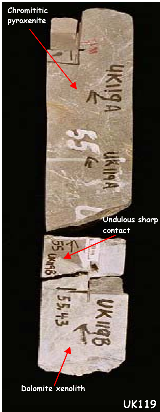
Figure 3. 17: Part of borehole core UK119, showing the undulous, sharp contact between the intrusive rocks (chromititic pyroxenite) and the dolomite xenolith.
