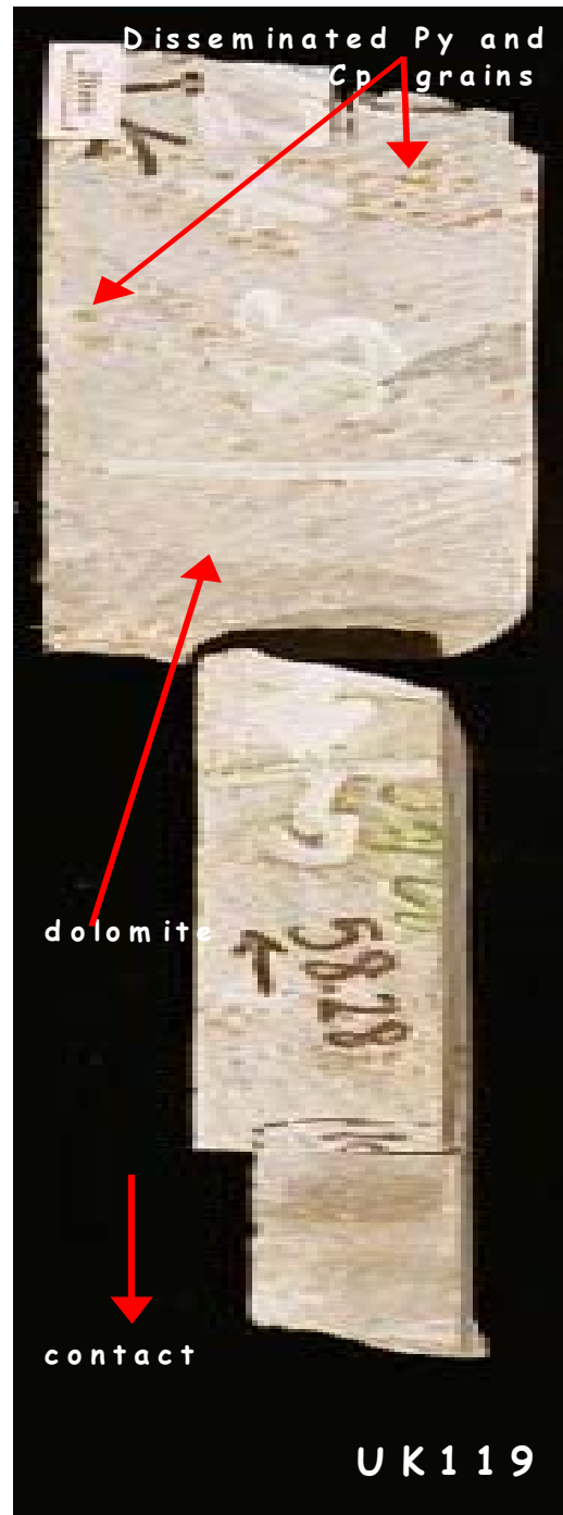
Figure 3. 18: Part of borehole core UK119, showing disseminated pyrite (Py) and chalcopyrite (Cp) grains in the dolomite xenolith close to the contact with the intrusive rocks.
