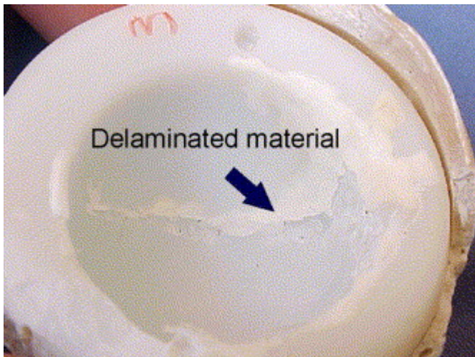
Fig. 3. Acetabular cup with delaminated material visible on inside of cup on bearing surface.
