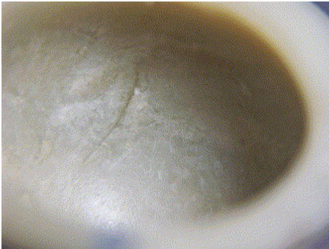
Fig. 10. Acetabular cup with severe scratches on inside.
