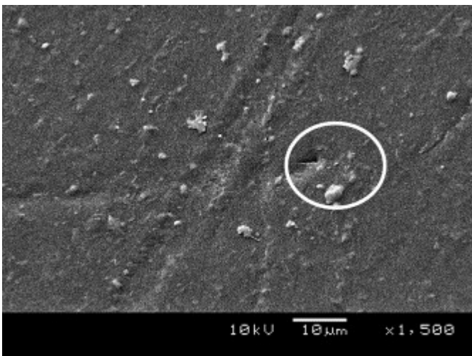
Fig. 16. Electron microscope back scatter analysis of scratch (magnification 1500×).
