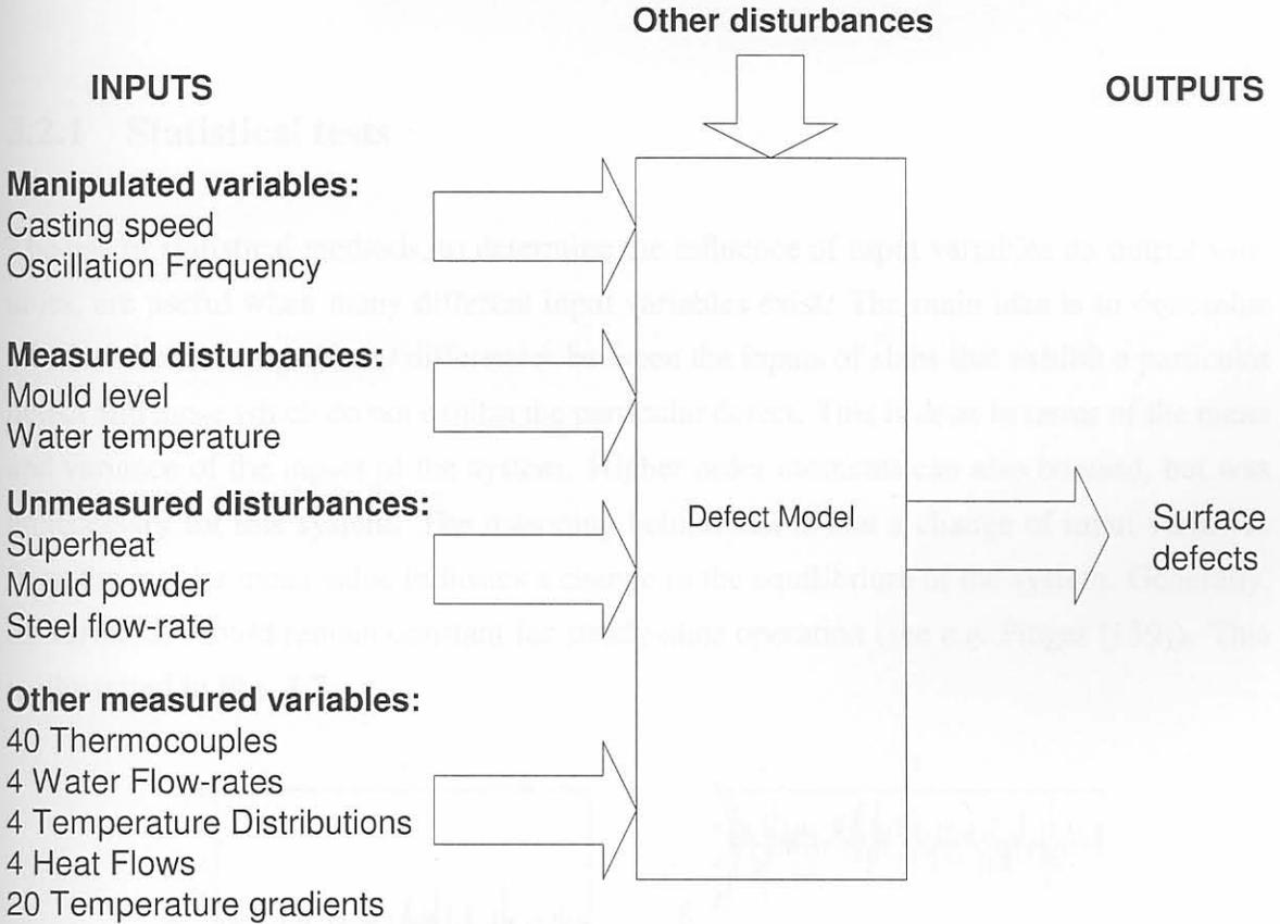
**Figure 3.6** Mould variables and defects in a system configuration.
