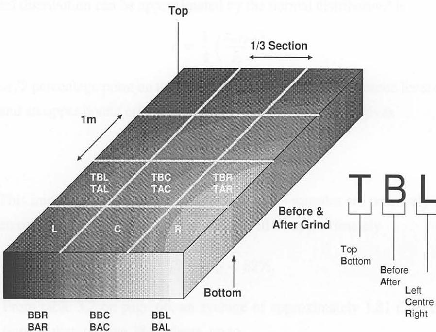
**Figure 3.4** Sub-division of the slabs into top and bottom; left, right and center; and before and after grinding. The casting direction is into the page.
