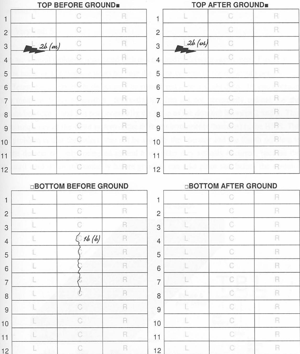
1a: transversal cracks, 1b: longitudinal cracks, 2a: casting powder entrapment, 2b other inclusions, 3: sticker, 4: bleeder, 5a: deep oscillation marks, 5b: uneven oscillation marks, 6: stopmarks, 7: footprints, 8: depressions.
