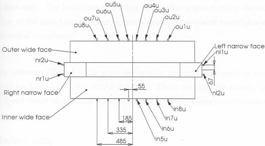
**Figure 3.2** Top view of the mould depicting location and naming conventions of the thermocouples. Note that in this view, the thermocouples shown are the top row of thermocouples. The bottom row of thermocouples have names “ou8l”, “nr1l”, etc.
