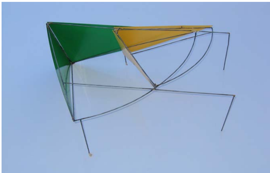
Figure 3.2.3a: A wire-model for the circular side failure-wedge when R_z \leq x < t .
