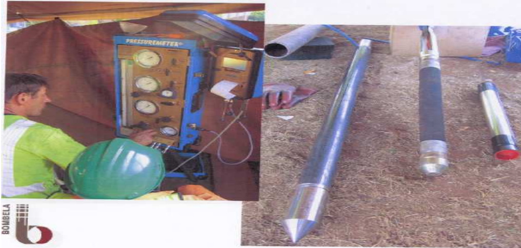
Figure 22: Pressuremeter Monitoring Box and expandable probe
