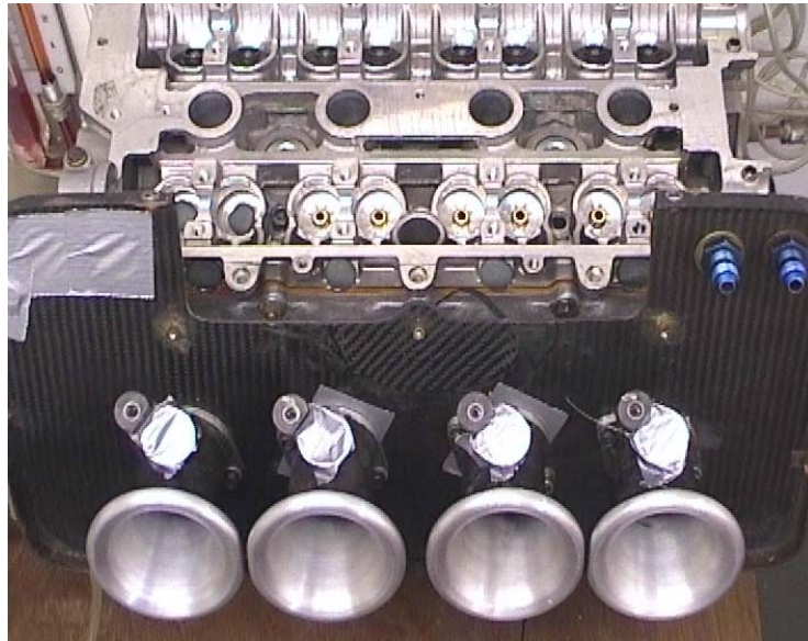
Figure C-3: Another view of trumpet and airbox base assembly
