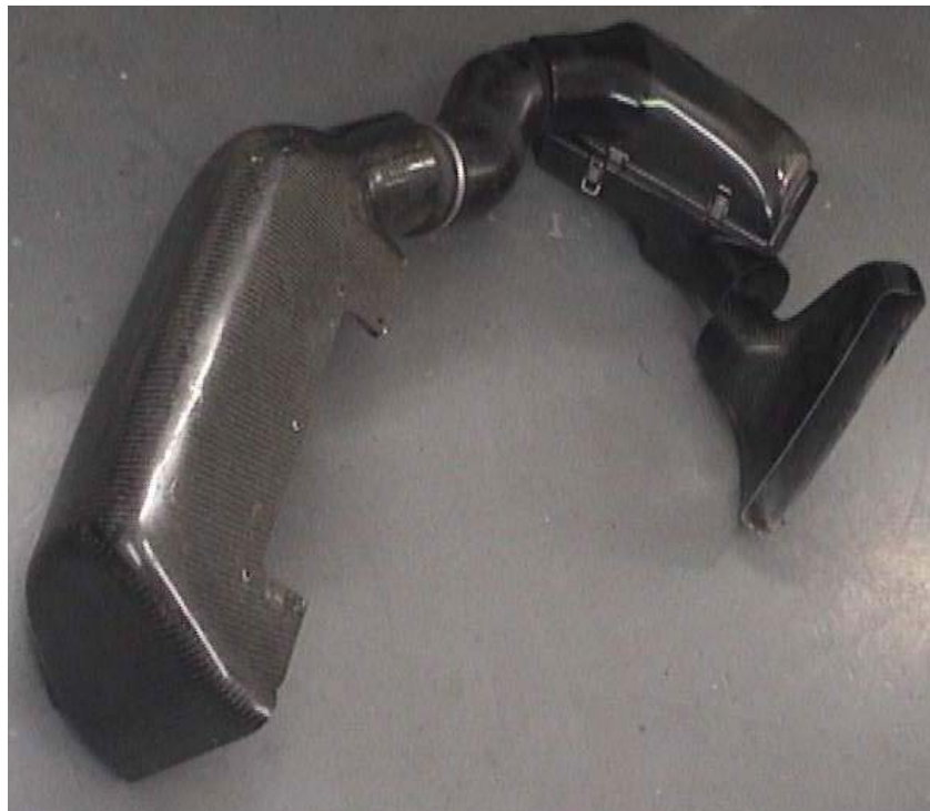
Figure A-5: Complete intake system
