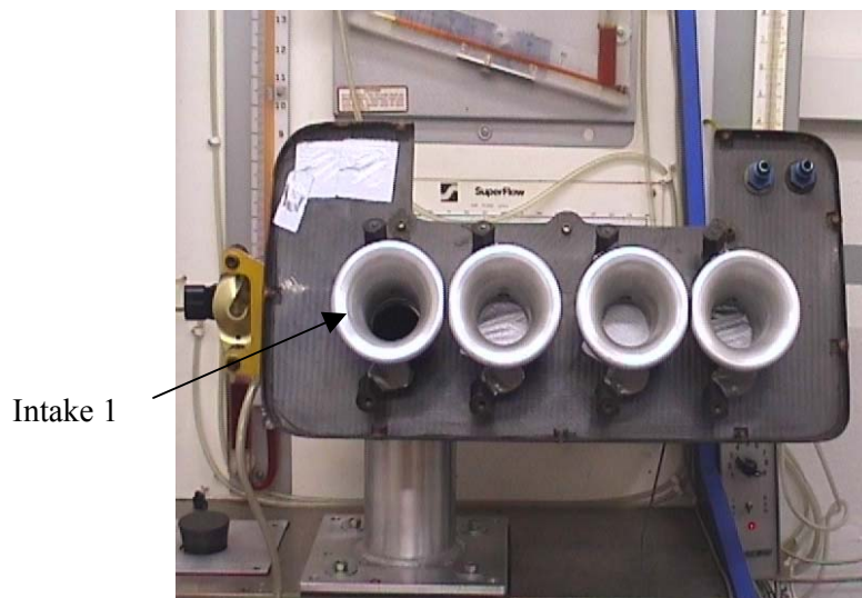
Figure C-2: Base of airbox with trumpets bolted on the cylinder head
