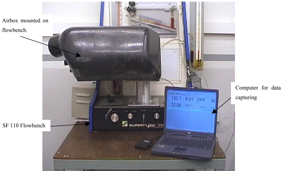
Figure 3-19: Flowbench experimental set-up
