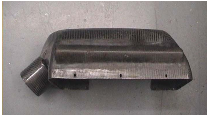
Figure A-1: Side view of airbox (firewall side)
