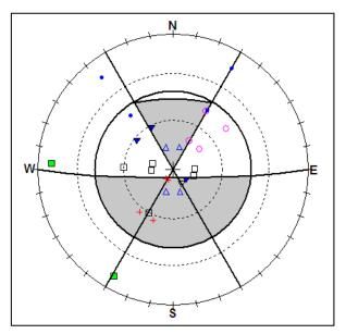
Figure 29: Toppling failure for a slope with dip direction of  $180^{\circ}$  and a dip of  $85^{\circ}$
