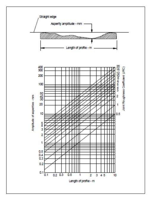
Figure 2: Alternative method for estimating *JRC* from measurements of surface roughness amplitude from a straight edge (Barton 1982).
