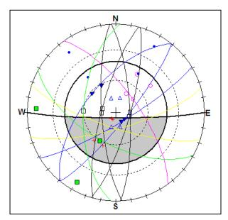
Figure 30: Wedge failure for a slope with dip direction of 180° and a dip of 85°
