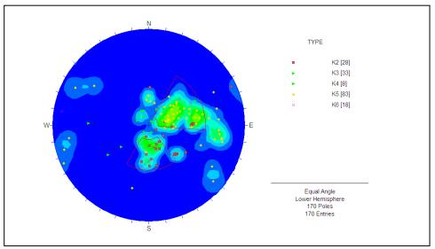
Figure 16: Stereo plot of foliation in the granitic gneiss
