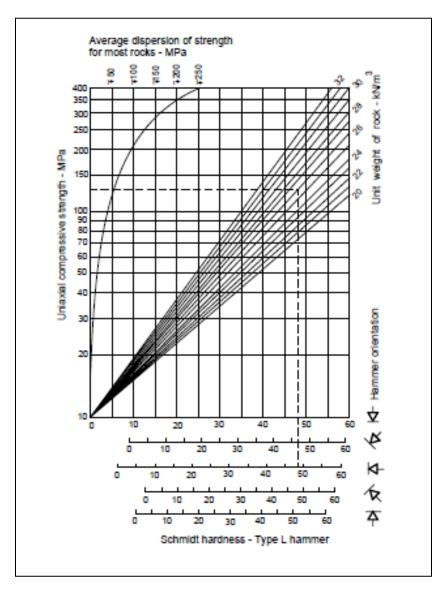
Figure 3: Estimate of joint wall compressive strength from Schmidt hardness. (Deere and Miller 1966)
