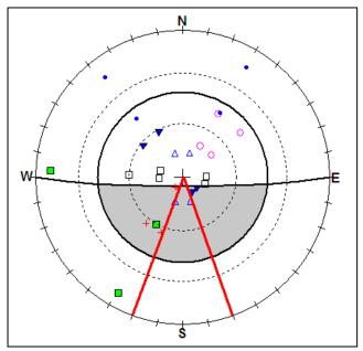
Figure 28: Plane failure for a slope with dip direction of 180° and a dip of 85°
