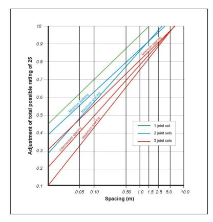
Figure 1 Graph for determination of joint spacing rating
