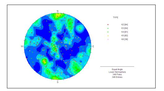
Figure 14: Stereo plot of joint patterns in the granitic gneiss
