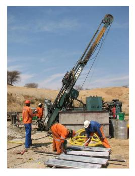
Figure 9: Drill rig drilling at -60°
