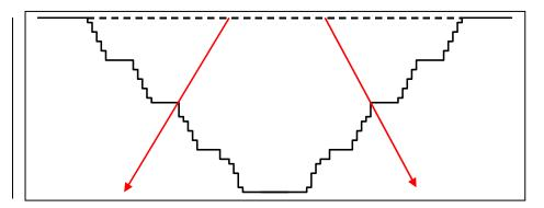
Figure 10: Schematic pit section indicating drill hole target areas
