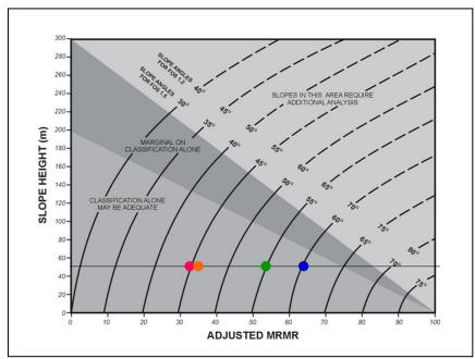
Figure 31: Slope design chart (Haines and Terbrugge, 1991) for BSA's
