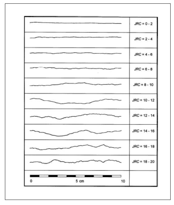
Figure 1: Roughness profiles and corresponding JRC values (After Barton and Choubey 1977).
