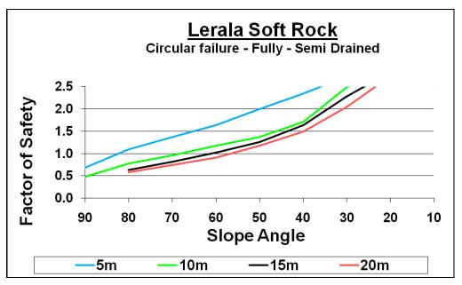
Figure 33: Slope angles and factors of safety for bench heights
