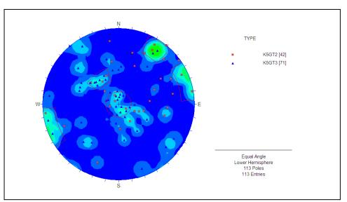
Figure 15: Stereo plot of joints in the K5 dolerite dyke
