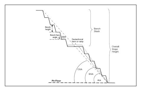
Figure 6: Open pit terminology SBW – Spill Berm Width ; OSA – Overall Slope Angle ; BSA – Bench Stack Angle ; IRA – Inter Ramp Angle
