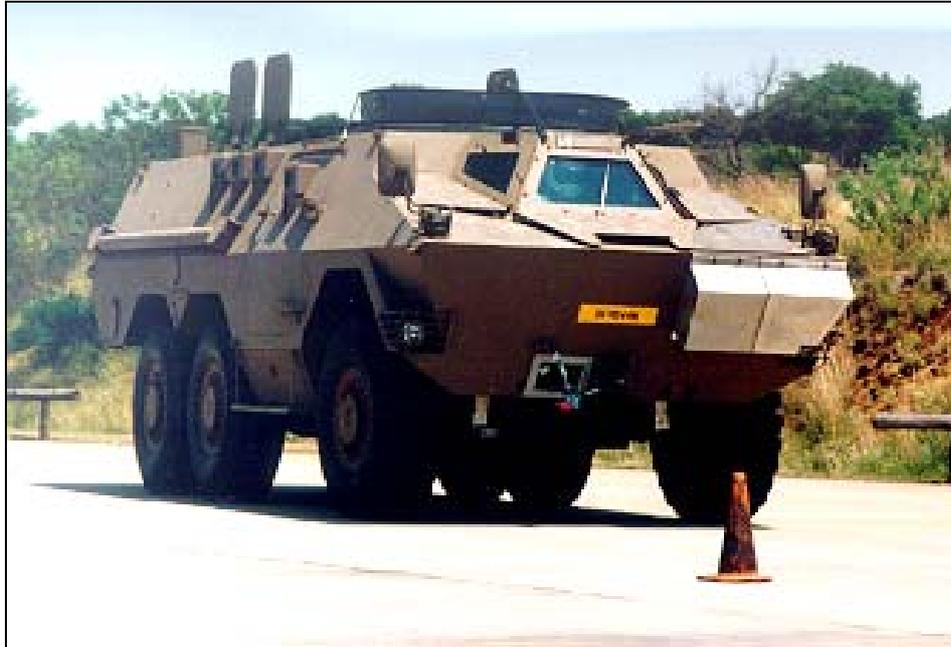
**Figure 1-5: 6x6 armoured personnel carrier fitted with semi-active dampers**
