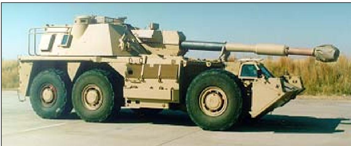
**Figure 1-7: GV6 self-propelled howitzer fitted with semi-active rotary dampers**
