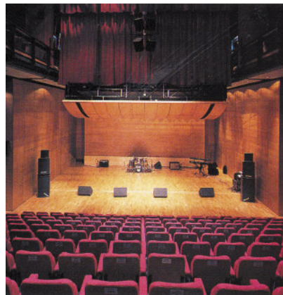
Fig 68. Back of screen acts as reflector
