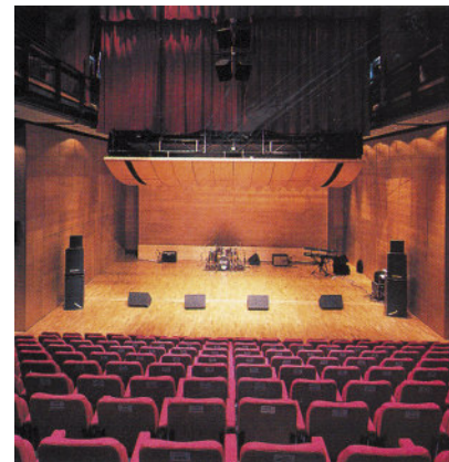
Fig 68. Back of screen acts as reflector
