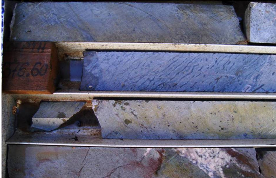
Figure 20: Proximal facies of GRAT showing erratic siliceous bedding and evaporitic textures and occurring fine grained replacement chalcopyrite. TCRD003-Tshifufia fragment.
