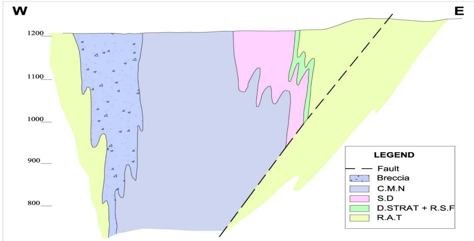
Figure 12: Section C-C' along the south part of the Tshifufia fragment. The known Roan breccias have outcropped in the eastern side of the mine. Small-scale folds are observed in the CMN strata. (Anvil Exploration, Houda B., 2008)
