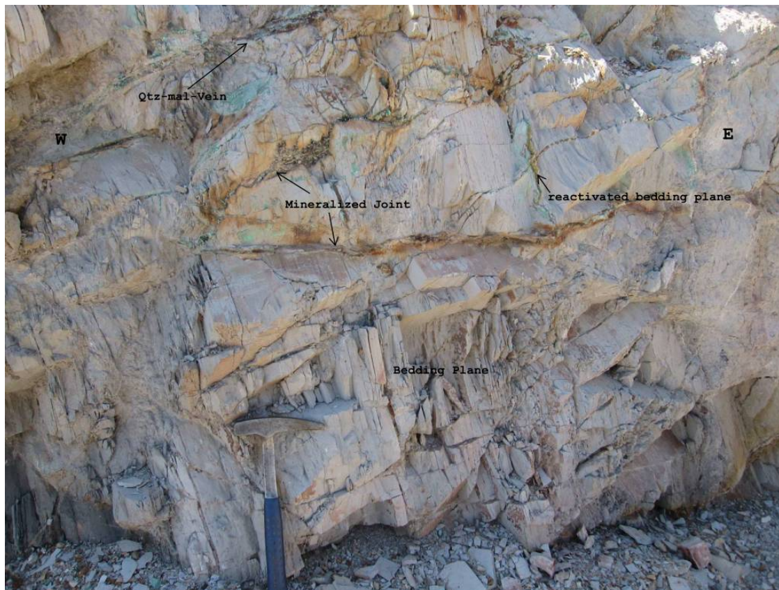
Figure 27: Open pit outcrop showing fractured SD with mineralised joint, Qtz-malachite veins and reactivated bedding planes – Tshifufia Fragment.
