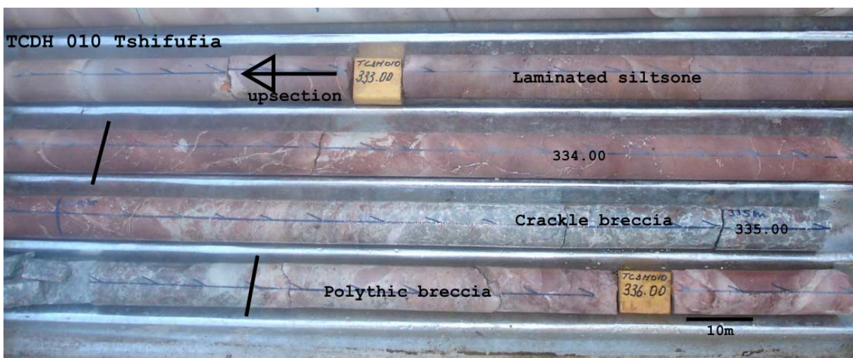
Figure 37: The contact between the crackle breccia and the heterogeneous breccia (RAT breccia).
