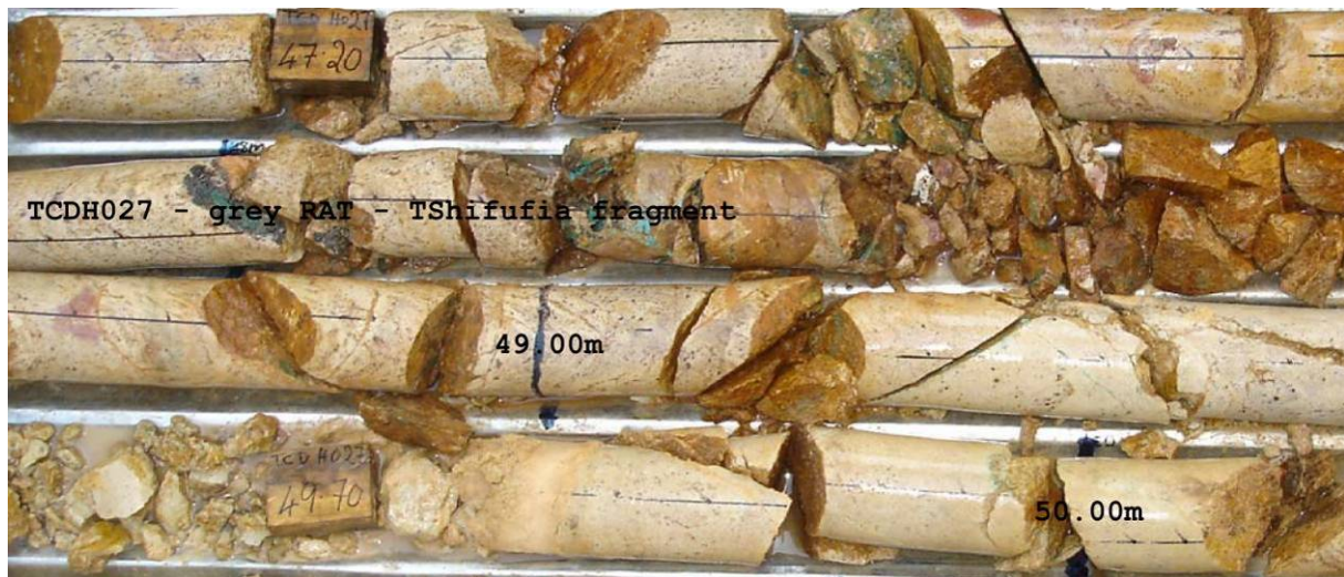
Figure 22: Yellowish-grey massive fractured dolomitic siltstone (Grey RAT) with hematite staining and malachite, heterogenite and manganese oxides in fractures (TCDH027-Tshifufia fragment).
