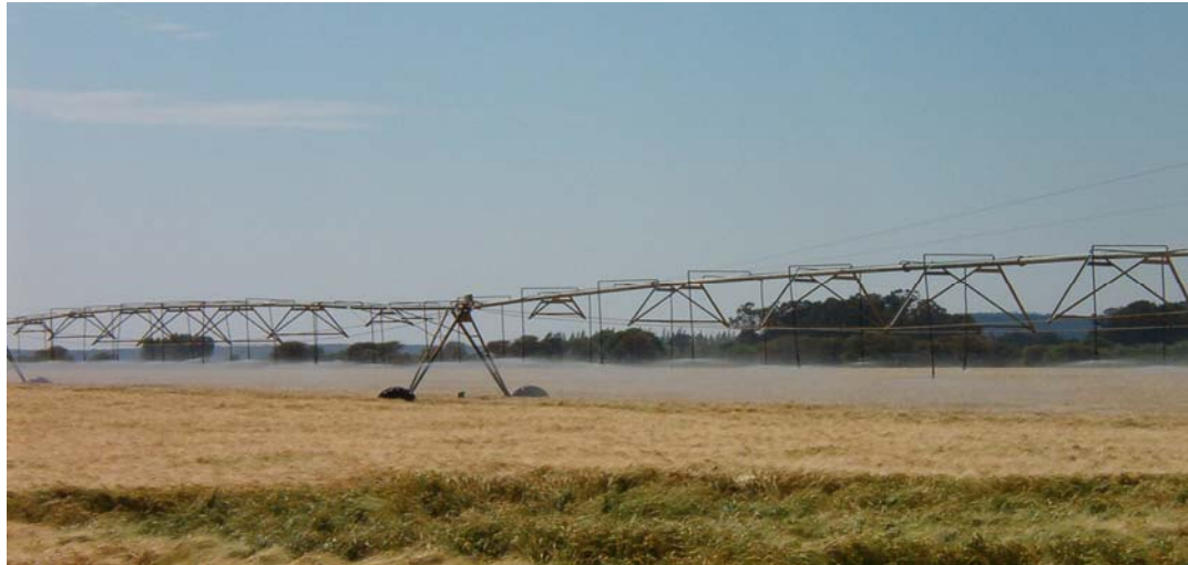
Photo 15. 1: Relative old and often under-designed centre pivot irrigation systems used for crop production at Taung Irrigation Scheme (2004)
