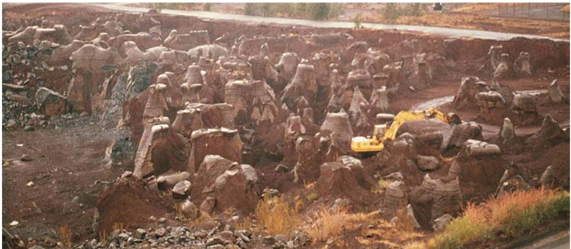
Plate 12. The variability of dolomite bedrock in the Lyttelton Quarry (I. Venter, 1981)
