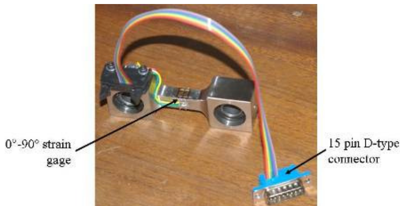
Figure 2.2. Uni-axial load cell used in the six component load cell
