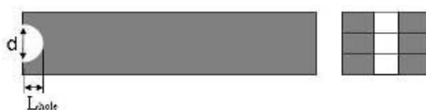
Figure B.19. Effect of hole on the area moment of inertia
