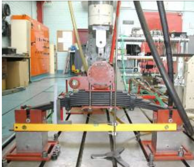
Figure 2.22. Experimental setup for measuring the deflection shape of the multi-leaf spring
