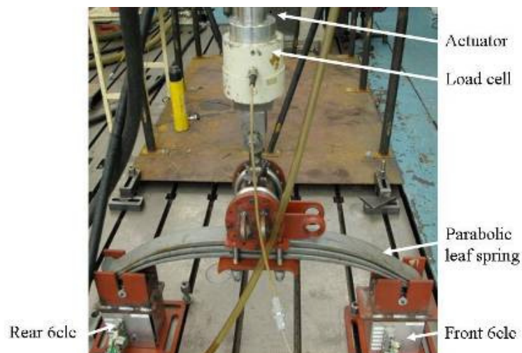
Figure 2.31. Experimental spring only setup of parabolic leaf spring
