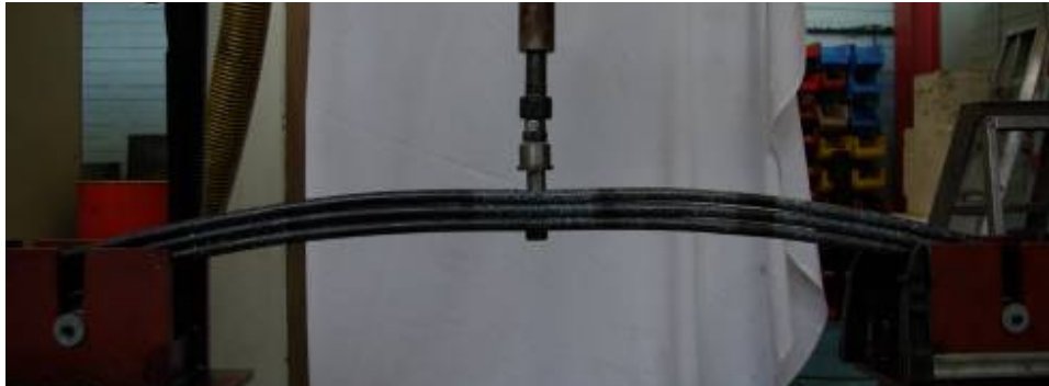
Figure B.17. Experimental setup of leaf spring with three full length blades and clamp length = 0m
