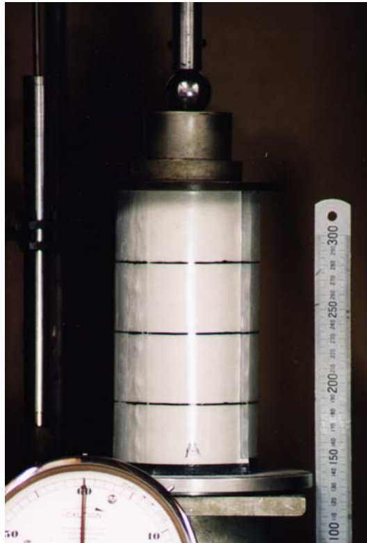
Figure 3.31 Single cell specimen in test machine.
