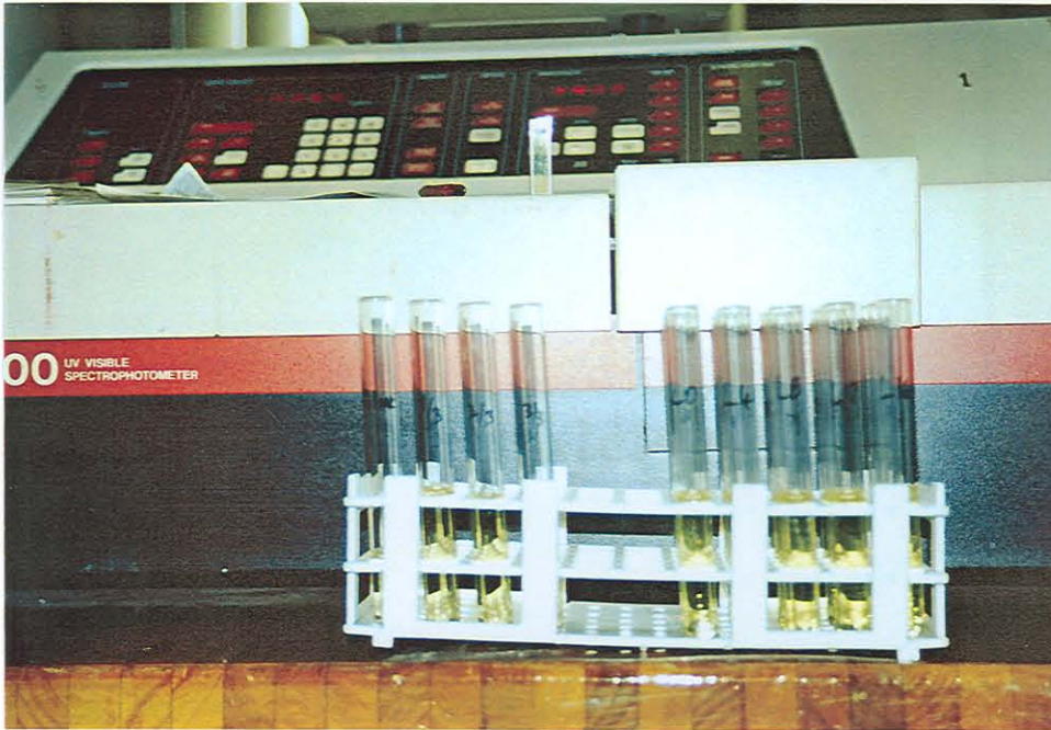
Plate 4 TNBS-PTA-FAN solutions and spectrophotometer
