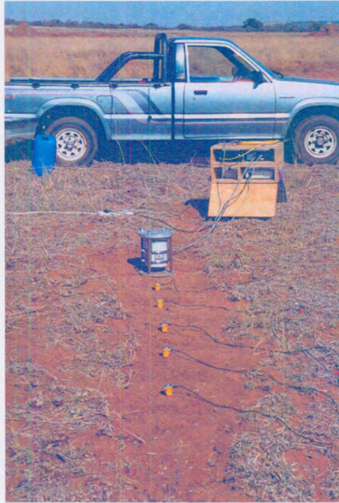
Figure 3.1 CSW testing prior to excavation (Test 1)
