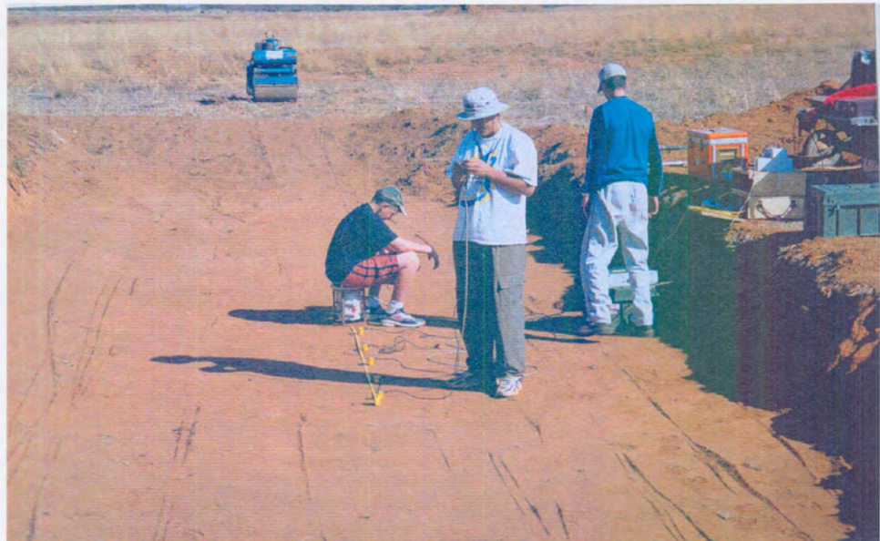
Figure 3.18 Preparing to perform CSW testing on second layer
