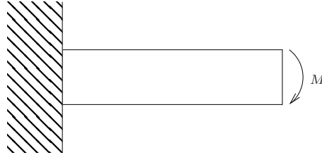
Figure 4.5: Cantilever beam in pure bending
