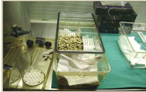
Figure 3.1: Tecniplast IVC cage with individual air supply (top removed, lying on the left).
