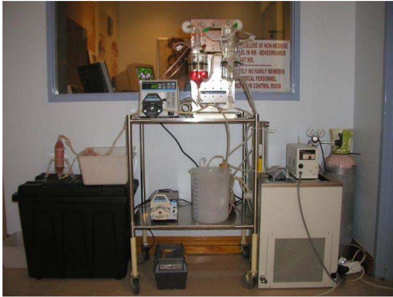
Figure 56: MRI experimental set-up showing numerous experimental components made from ferrous materials
