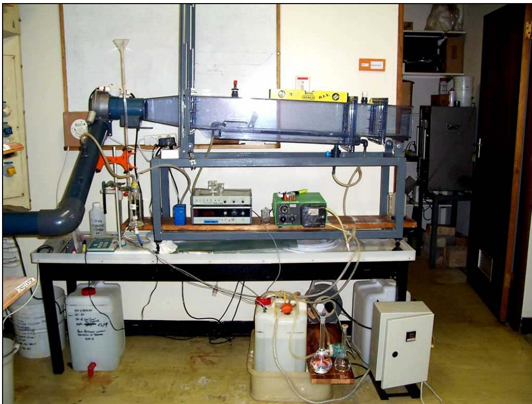
Figure 7.4. Photo of wind tunnel apparatus used to measure mass transfer coefficients.
