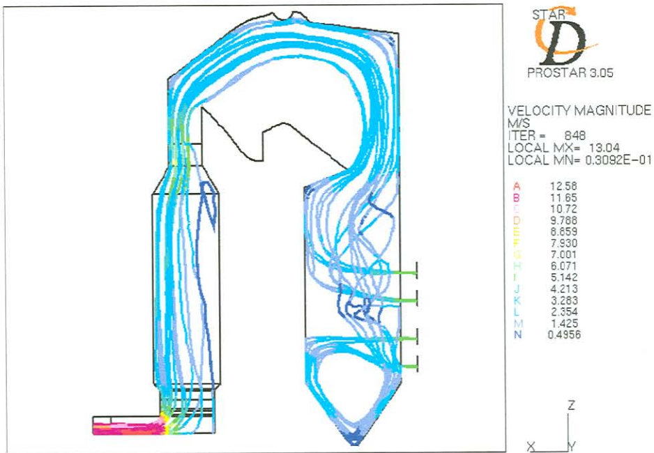
Figure 4-20 Particle Trajectories for 10 \mu m Particles
