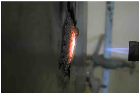
With no coating: Left top – 30 sec exposure Right top – 50 sec exposure Left and right bottom – 80 sec exposure
