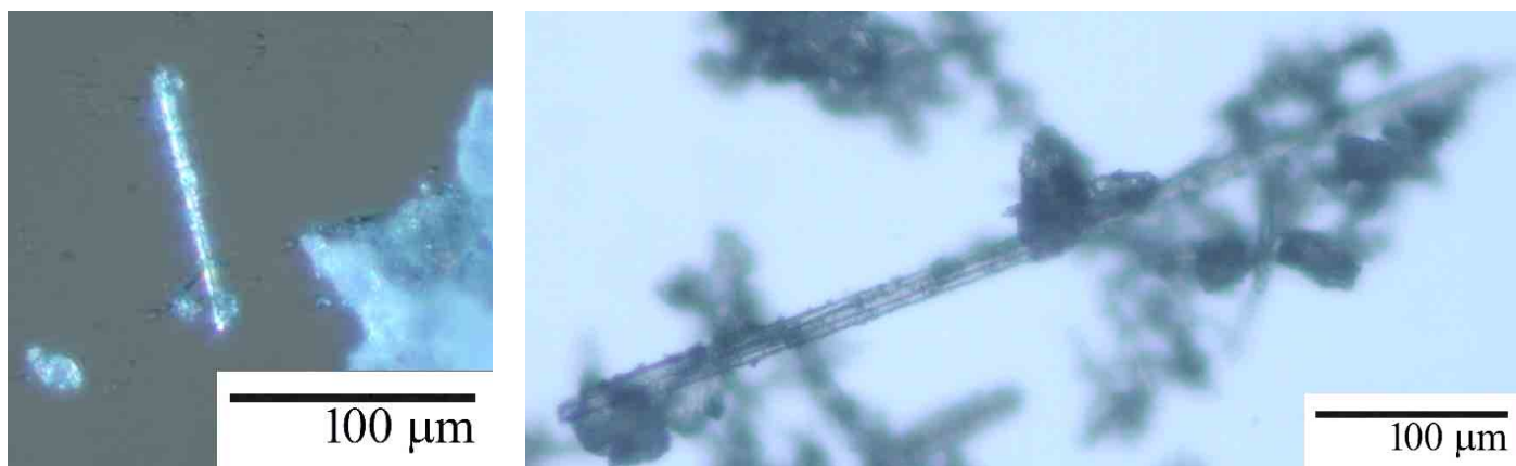
Light microscope images of calcium gluconate monohydrate crystals (powder)
