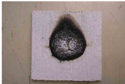
With Gluconate/silica/graphite coating: Left top – 60 sec exposure Right top – 270 sec exposure Left and right bottom – 360 sec exposure
